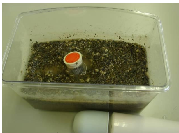
Fig.1 Liquefaction experiment by water tank and portable massager explaining uplifting the manhole.
